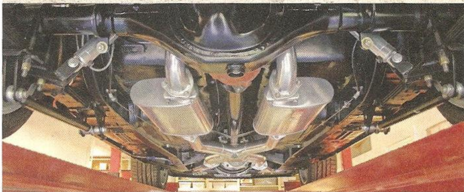
Undercarriage of this Boss is as clean and meticulous as topside, including custom 2.5-inch exhaust
