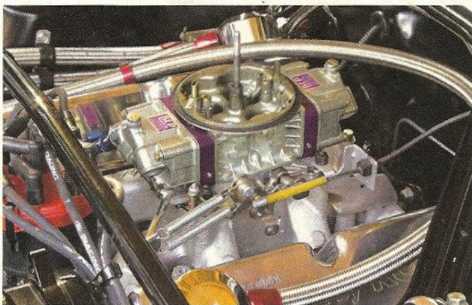
Race-prepped BLP carburetor mounted to Edelbrock Victor Jr. intake feeds Roush engine; Hydratech makes the hydraulically powered brake booster
