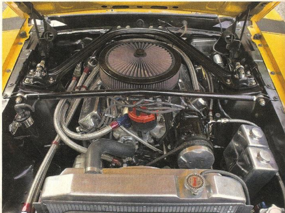
KRC pump feeds power steering and brakes; Roush 342-cu.in. crate engine makes broad, reliable power band while original Boss 302 sleeps safely
