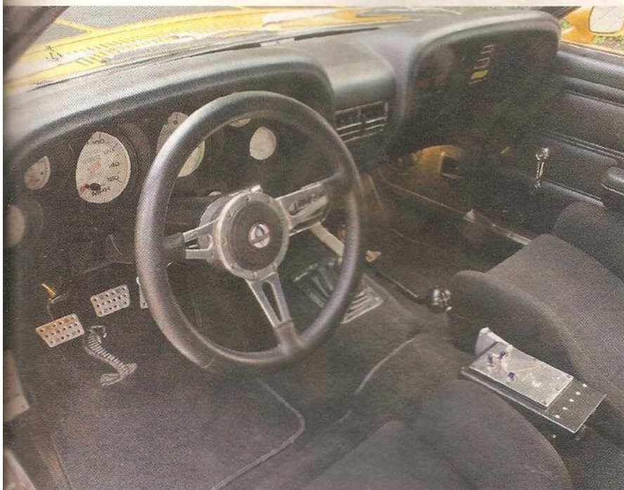
Auto Meter gauges reside in stock dash, rally timer gear mounts to passenger side; long shift handle bridges distance from Corbeau seats to five-speed
